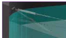
Mooring cables with springs and wall brackets
